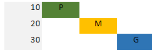
Fig. 5. Linguistic variables for concentration of ceramic particles Al 2 O 3 in bath (g/l)
