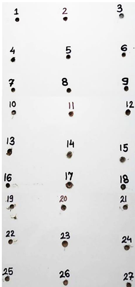
Fig. 5. Experimental Results after ECDM Drilling
