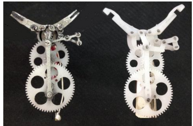
Fig. 1. Flapping mechanism fabricated through EDM (Al 7075) and injection moulding (POM)
