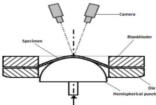
Fig. 1. Basic schema of Nakazima test, [2]
