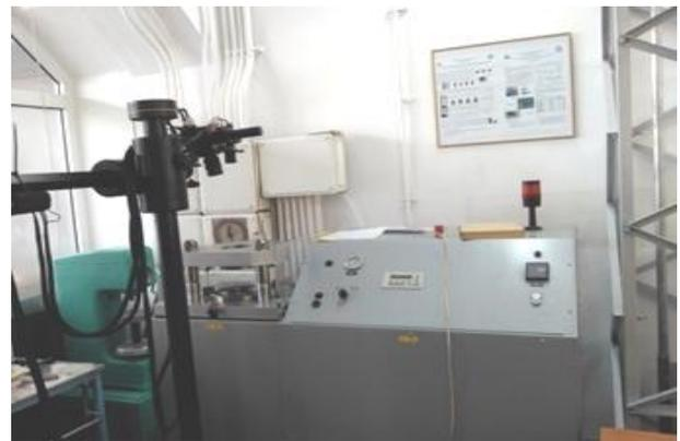
Fig. 2. Testing installation for Nakazima test
