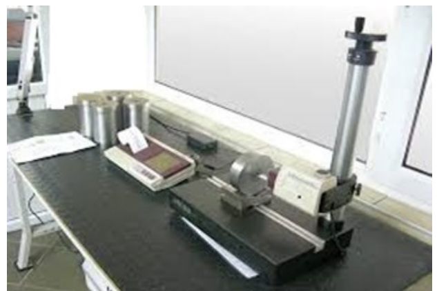
Fig.5. Measurement of surface roughness
