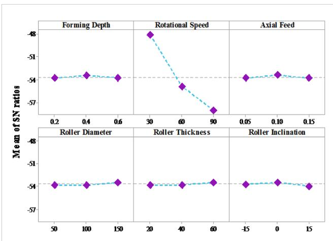
Fig.7. Graph of S/N ratio of Circumferential Force
