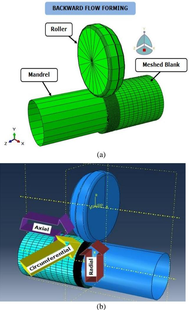
Fig.2. (a) initial 3D model with meshed blank (b) forces acting during the process
