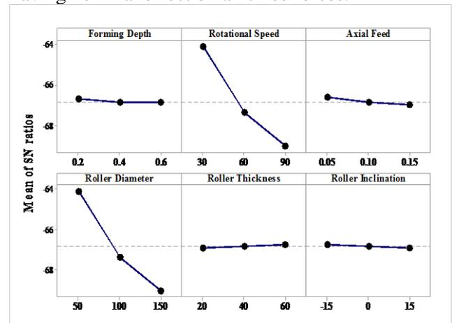
Fig.5. Graph of S/N ratio for Axial Force
