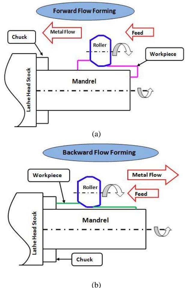
Fig.1. Schematic diagram of flow forming (a) Forward (b) Backward
