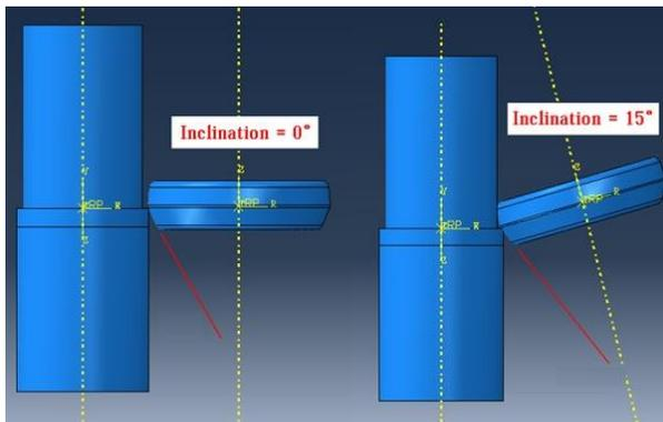
Fig.4. Roller inclination with workpiece
