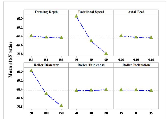
Fig.9. Graph of S/N ratio of Resultant force
