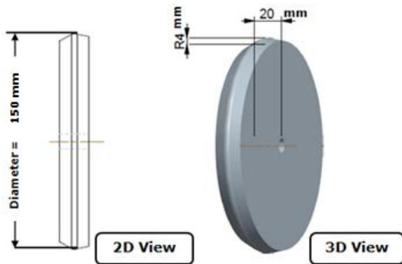
Fig.3. Roller diameter and thickness
