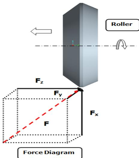
Fig.8. Resultant force Diagram
