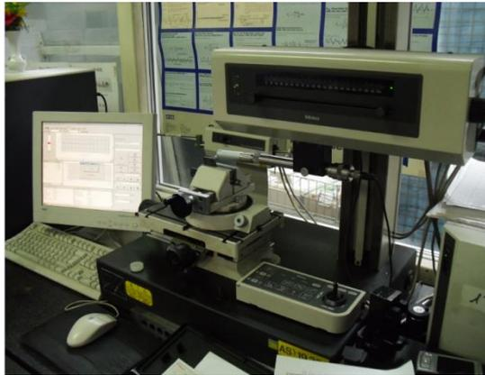
Fig. 2. Roughness measuring equipment
