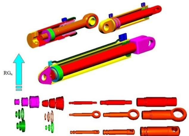
Fig. 6. A modular system of hydraulic cylinders (Gendarz, 2009)
