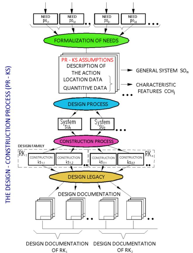
Fig. 2. The design construction process of creating the design family (Gendarz, 2009)
