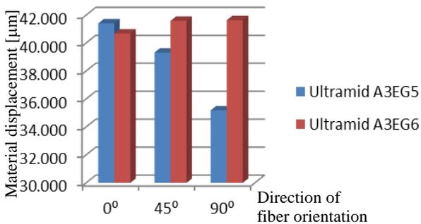
Fig. 5. Material displacement
