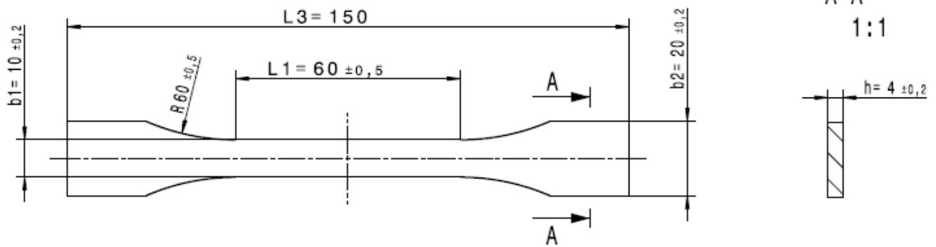
Fig. 1. Specimen dimensions according to ASTM D638-02
