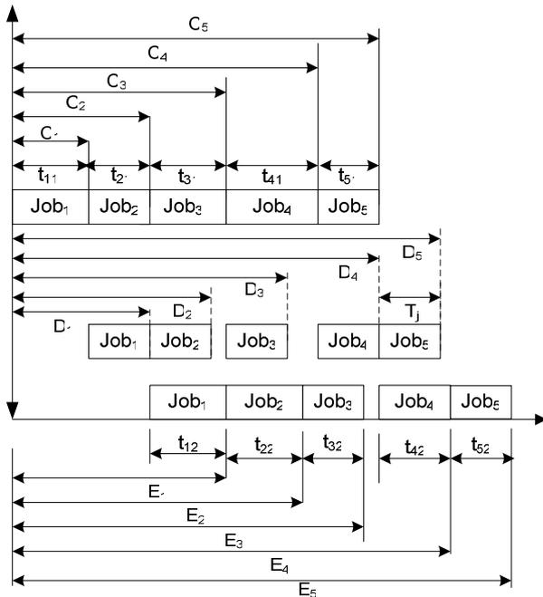
Fig.1. Completion time, delivery time to  $M_2$  and end time of jobs
