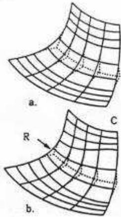
Fig.3. Law of free surfaces: a - constant; b - variable; R - radius
