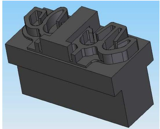
Fig.12. The 3D model of the electrode for finishing
