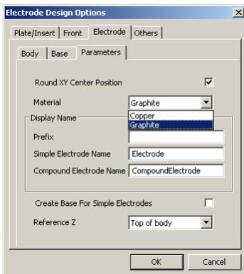
Fig.10. Specification of the electrode material
