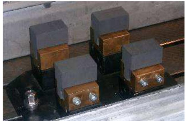
Fig.13. Modular device with four clamping elements, mounted on the table of machine FADAL VMC2216
