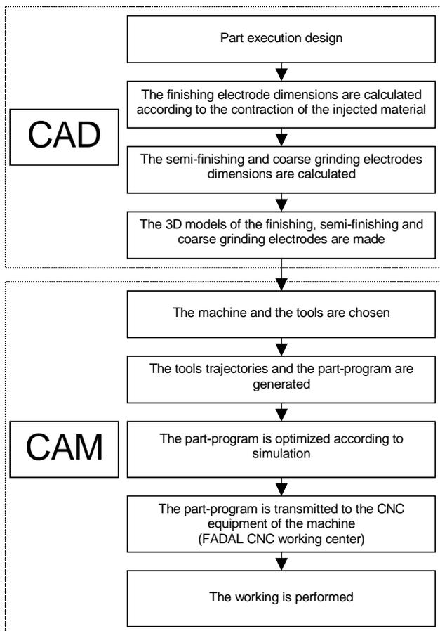
Fig.7. Principle of the electrodes realization
