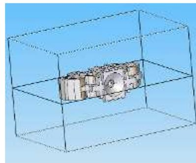
Fig.9. The semi-molds (without the cylindrical core) for the plastic part to be made
