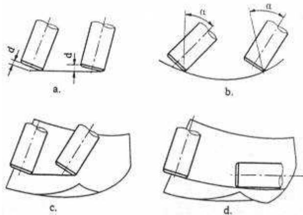
Fig.4. Milling geometry for 5-axes milling with frontal mill: a – constant  $d$  distance; b – constant  $\alpha$  angle; c – maximum tool-part contact; d – NC rolling (flank processing)
