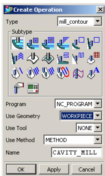
Fig.17. Selection of milling type
