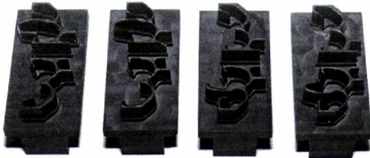
Fig.21. Ready made electrodes
