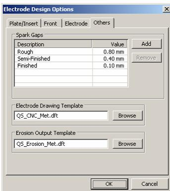
Fig.11. Specification of the electrode parameters
