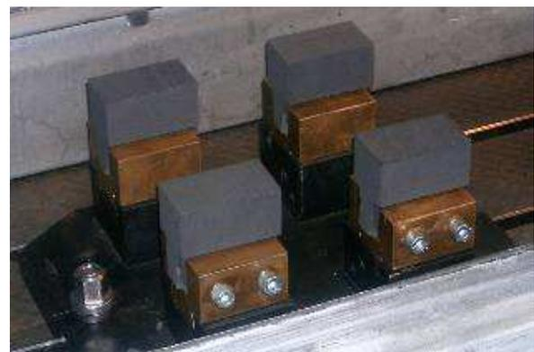
Fig.19. Modular device with four clamping elements, mounted on the table of machine FADAL VMC2216
