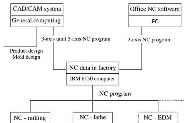
Fig.1. Integrated CAD/CAM systems for mold realization
