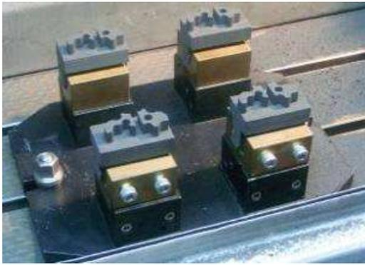
Fig.20. Roughly trimmed electrodes
