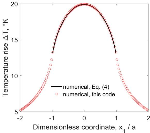
Fig. 2. Temperature rise due to a circular heat source,  $\dot{H} = 0.2\pi\text{W}$ ,  $K = 50.2\text{W}/(\text{m}^\circ\text{K})$ ,  $a = 0.2\text{mm}$ .
