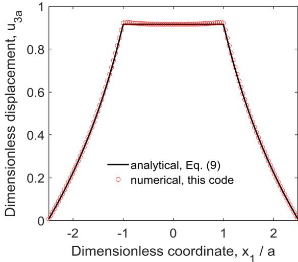
Fig. 3. Thermoelastic distortion due to a ring heat source.
