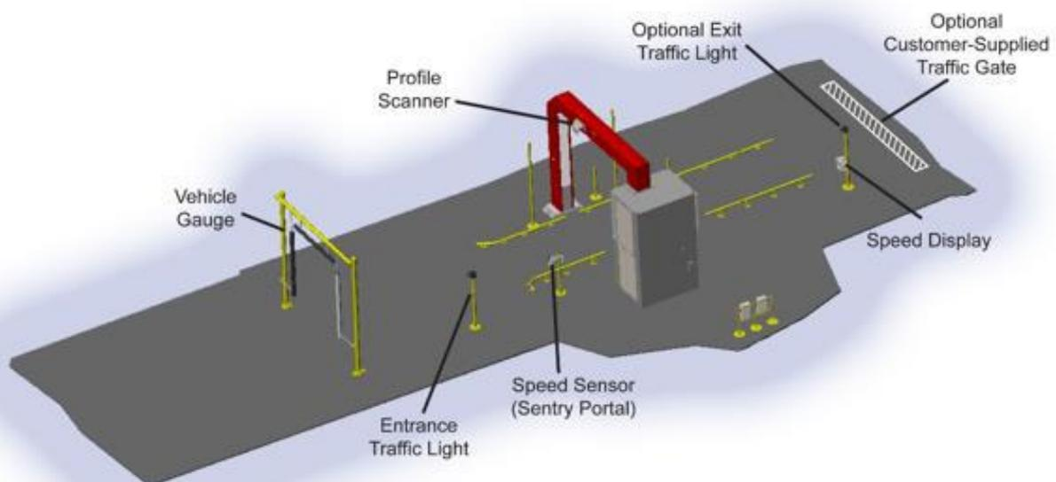
Fig. 10. Cargo Inspection Portal System, [13]
