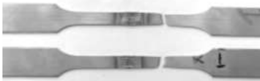
Fig. 16. Samples of joint I after static tensile test.
