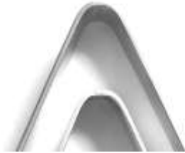
Fig. 13. Samples of joint I after bending test.
