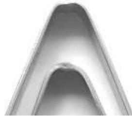
Fig. 15. Samples of joint III after bending test.
