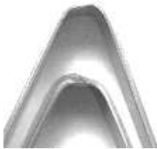
Fig. 14. Samples of joint II after bending test.
