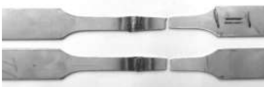
Fig. 17. Samples of joint II after static tensile test.
