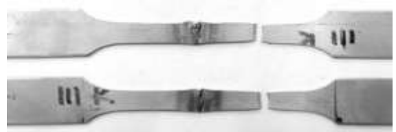
Fig. 18. Samples of joint III after static tensile test.
