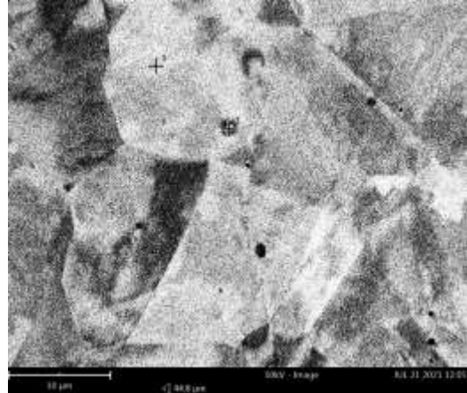
Fig. 23. SEM image of microstructure of the HAZ of single-welded non-melted joint (I).
