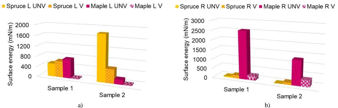
Fig. 5. Comparison between surface energy in accordance with different samples: a) samples cut in longitudinal direction; b) samples cut in radial direction
