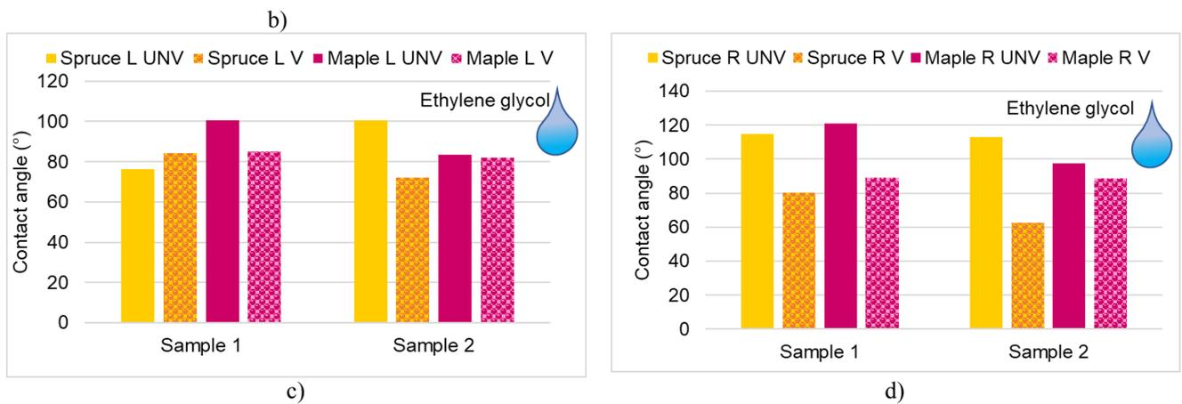
Fig. 4. Variation of contact angle in accordance with different samples: a) samples cut in longitudinal direction, water drop; b) samples cut in radial direction, water drop; c) samples cut in longitudinal direction, ethylene glycol drop; d) samples cut in radial direction, ethylene glycol drop
