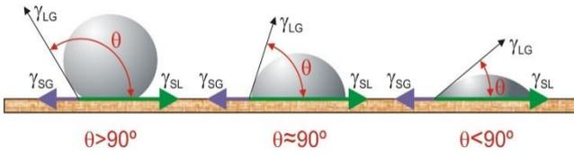
Fig. 2. The measurement of the contact angle [7, 8]
