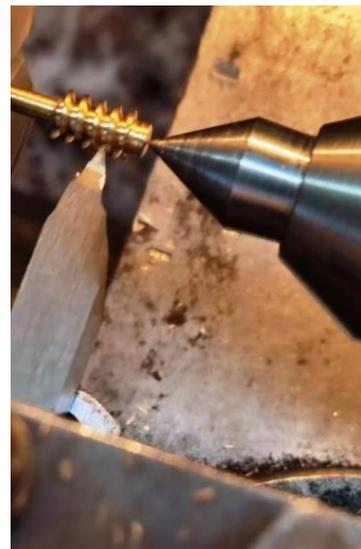
Fig. 4. Turning the worm prototype
