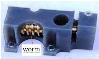
Fig. 6. Test the worm gear machined prototype
