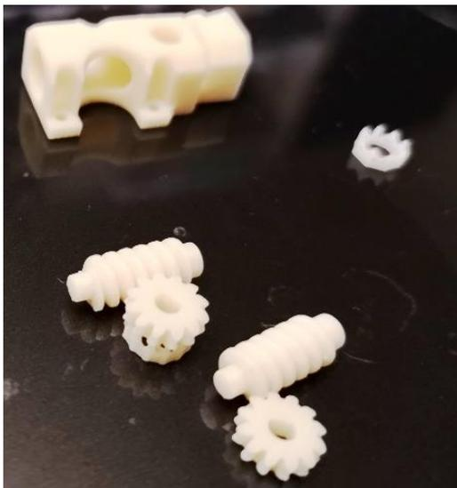
Fig. 3. 3SP printed parts
