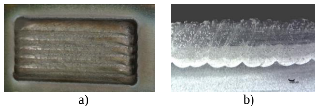
Fig. 9. Structure of the three-layer overlay weld: a) face, b) overlay weld macrostructure; substrate – steel S355, overlay weld I: 95% Inconel 625+5% WC, overlay weld II: 90% Inconel 625+10% WC and overlay weld III: 85% Inconel 625+15% WC
