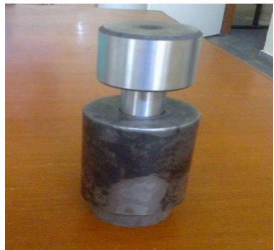
Fig. 1. Photograph of the die used to prepare compacts
