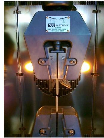
Each tensile test was performed on the segment no. 4 being positioned at the middle of the rod. Therefore, the A<sub>2</sub>-test is missing because the failure of the sheath occurred exactly across the segment no. 4 when drawing was actually unfinished.
