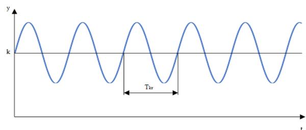
Fig. 10. System brought to the limit of stability
