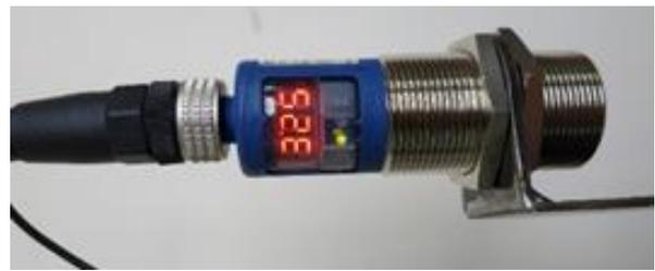
Fig. 6. Ultrasonic position sensor
