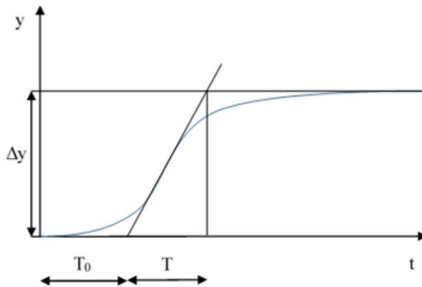
Fig. 7. Step response of the inertial system
