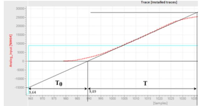
Fig. 8. The open system response in the Ziegler-Nichols method
