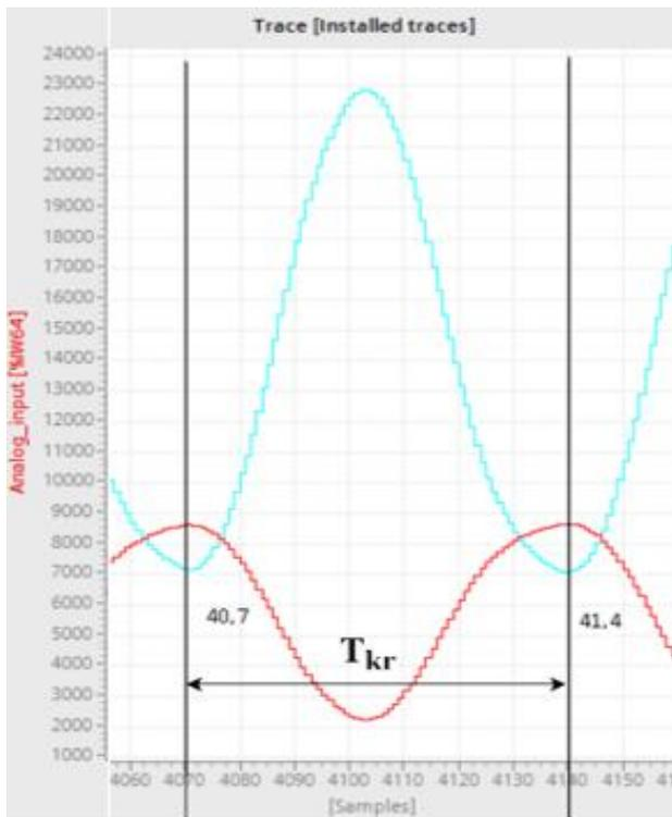
Fig. 11. Critical vibrations during the II Ziegler-Nichols method
