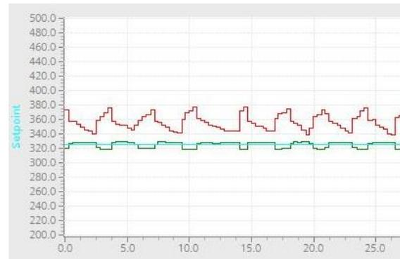
Fig. 9 Obtained the first result of the adjustment Ziegler - Nichols
