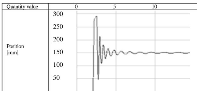
Fig. 15. The simulation result for the settings obtained by the manual tuning method
