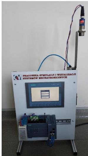
Fig. 4. Stand for testing the selection of the adjustment parameters of the pneumatic actuator
