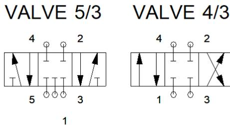
Fig. 1. Diagrams of valves that allow stopping the actuator position [9]
