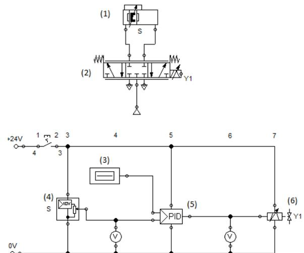
Fig. 13. The circuit diagram made in FluidSIM-P
