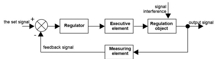
Fig. 3. Diagram of the regulator's operation
