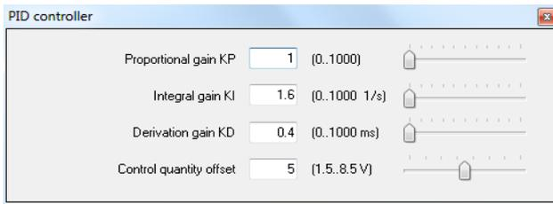
Fig. 14. Parameter window of the PID controller with final settings
