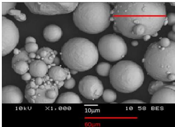
Fig. 1. SEM image of Ti6Al4V powder
