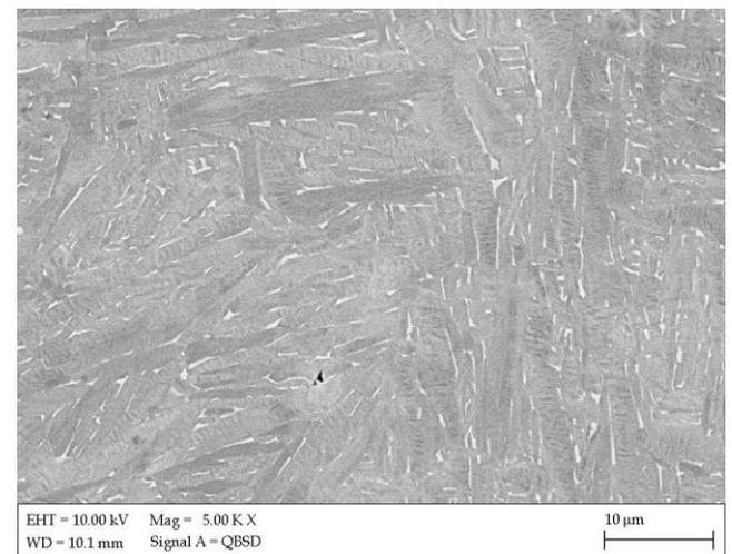
Fig. 9. The Microstructure of Ti6Al4V alloy, SEM
