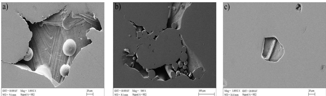
Fig. 5. Example results of microscopic observation SEM, a) lack-of-fusion pores, b) binding effect, c) gas pore
