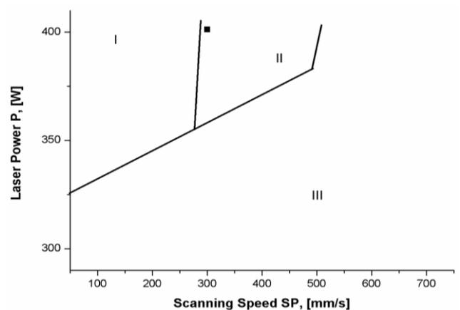
Fig. 7. Windows of parametres for the Ti6Al4V components manufactured by SLM/SLS process; I - melting with the cracks or porosity, II – full melting, III - partial melting
