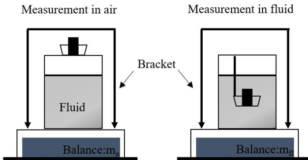
Fig. 2. Schematic of the Archimedes method for density measurement
