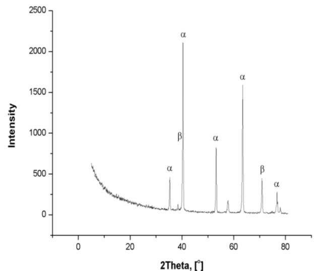
Fig. 10. X-ray diffraction pattern of investigated alloy
