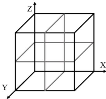
Fig. 3. Geometry of the tested samples with positions of the micro CT samplecut in the YX and XZ planes
