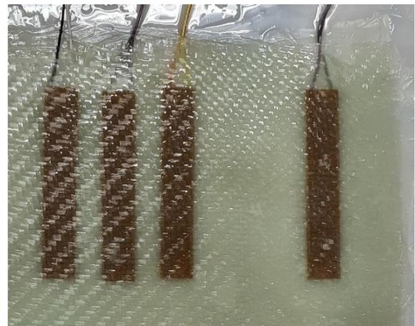
Fig. 7. A ready-to-use composite panel containing MFC piezoelectric transducers
