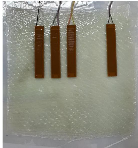
Fig. 6. Piezoelectric transducers during the process of lamination between the 3rd and 4th layers of glass fiber cloth
