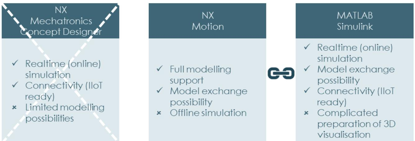
Fig. 2. Characteristics of available simulation tools
