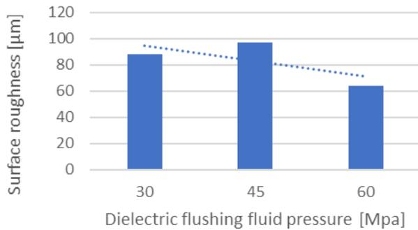
Fig. 9. Influence of dielectric flushing fluid pressure on the surface roughness of the workpiece
