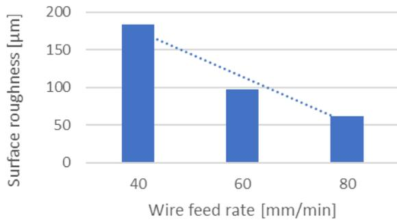
Fig. 10. Influence of the wire feeding speed on the surface roughness of the workpiece
