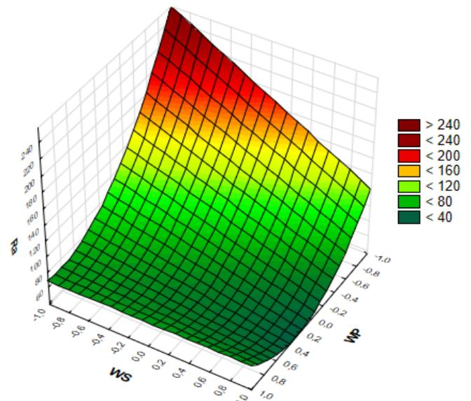
Fig. 5. Influence of wire rewinding speed WS and flushing fluid pressure WP on surface roughness Ra at an average head feed rate
