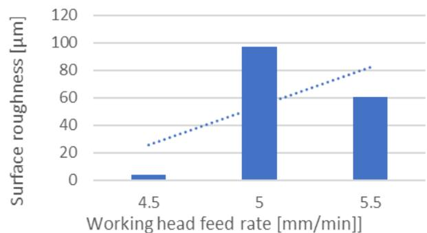
Fig. 8. Influence of the working head feed rate on the surface roughness of the workpiece
