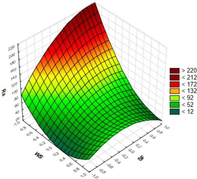
Fig. 6. Influence of wire rewinding speed WS and head feed rate SF on surface roughness Ra at an average flushing fluid pressure
