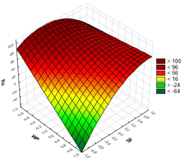
Fig. 7. Influence of flushing fluid pressure WP and head feed rate SF on surface roughness Ra at average wire rewinding speed
