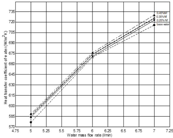
Fig. 12. Variation of heat transfer coefficient of water in annular with water mass flow rate for different volume
