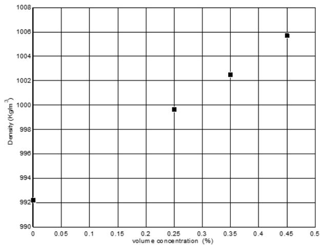
Fig. 8. Effect of nano-particle concentration on the density of nano-fluid
