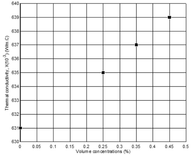
Fig. 5. Effect of nano-particle concentration on the thermal conductivity of nano-fluid
