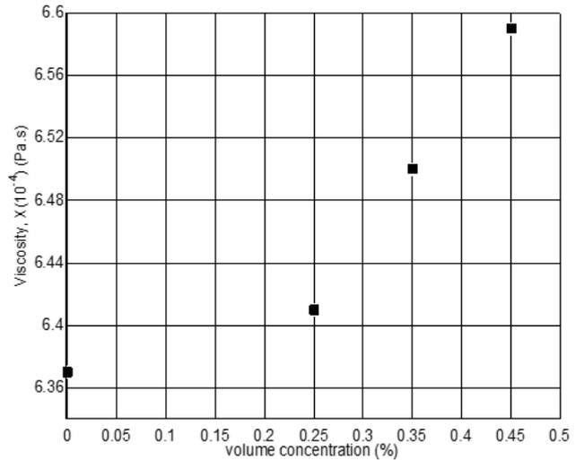
Fig. 6. Effect of nano-particle on the viscosity on nano-fluid
