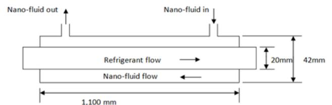
Fig. 4. The test section
