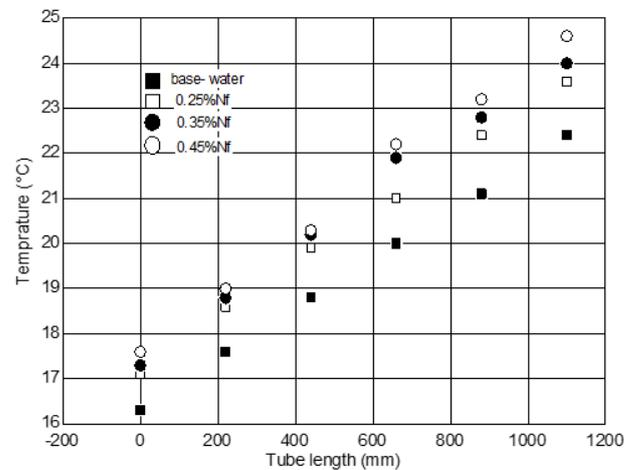
Fig. 10. Temperature distribution along tube heat exchanger refrigerant side
