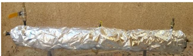
Fig. 3. Evaporator heat exchanger with insulation
