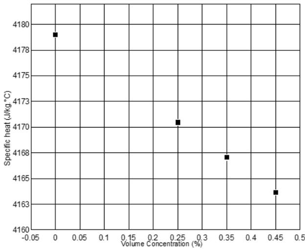
Fig. 7. Effect of nano-particle concentration on the specific heat of nano-fluid
