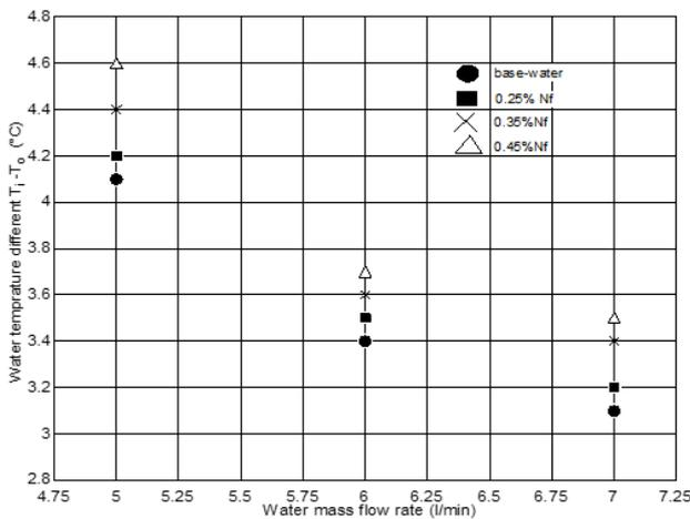
Fig. 13. Effect of water mass flow rate on the water Temperature difference with base refrigerant
