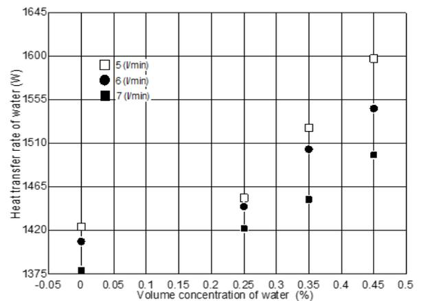
Fig. 11. Effect of volume concentration on heat transfer rate with water mass flow rate
