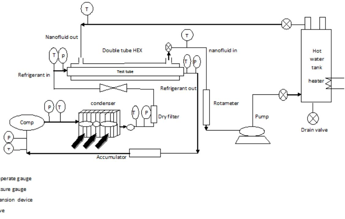
Fig. 2. Schematic diagram for the experimental test rig
