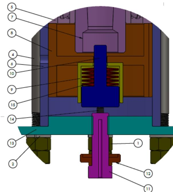
Fig. 3. Detailed section view of testing device
