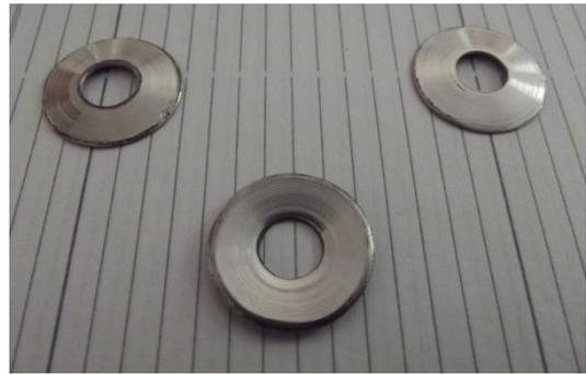
Fig. 4. Shape memory alloy disc springs used in the device
