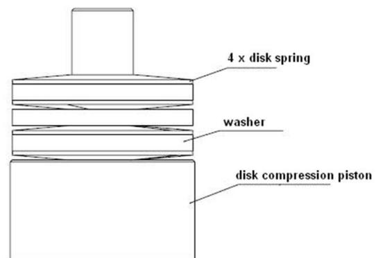
Fig. 8. The 4 memory shape disks in bearing preload arrangement
