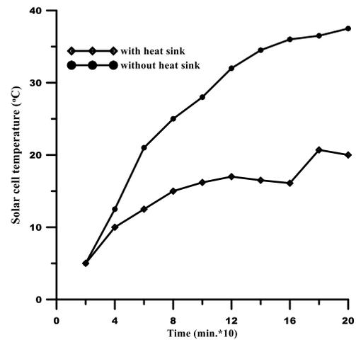
Fig. 4. The solar cell temperature versus operation time
