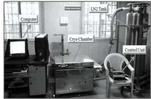
Fig. 2. A typical representation of cryogenic treatment process
