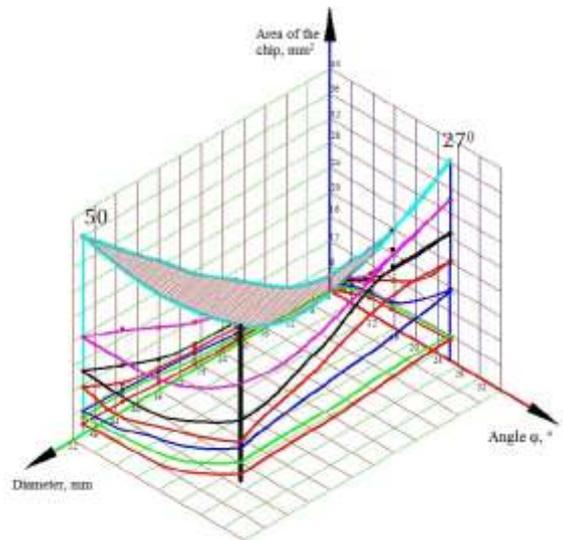
Fig.6. Changing the chip area depending on the angle  $\varphi$  and the diameter of the milling cutter D
