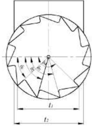
Fig.2. Central angles defining the position of the teeth of the milling cutter
