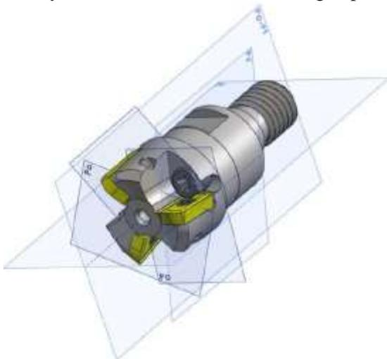
Fig.5. Non-monolithic milling tool with three carbide cutter insert
