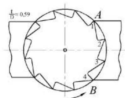
Fig.4. Scheme for determining the simultaneously working teeth
