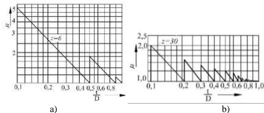
Fig.3. Graphical representation of changing of  $\mu$  depending on the number of teeth of the milling cutter  $z$
