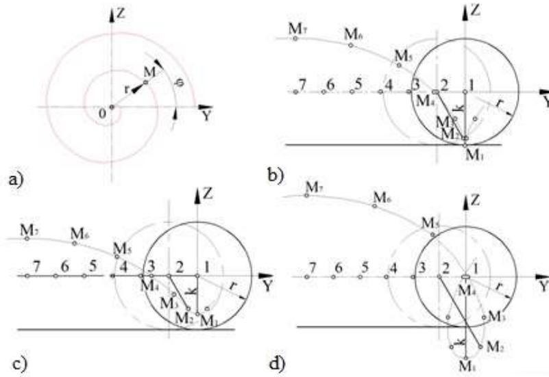
Fig. 1. Relative milling trajectories
